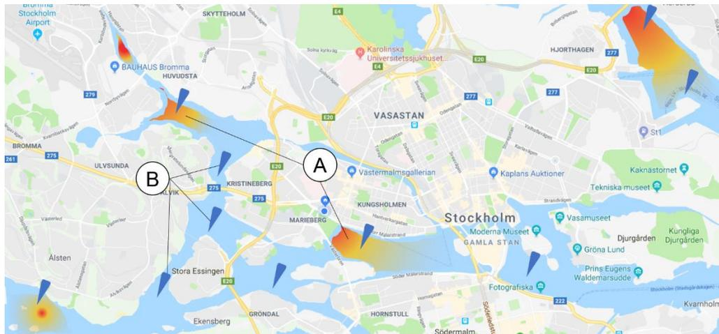
**Figure 3.** Example of how the visualization of the water monitoring solution could be developed, where the red areas (A) are potential pollution. The blue pointers (B) are sensors in the network.
