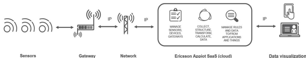
**Figure 2.** High level architecture for the technical set-up of data catchment from sensors to cloud and visualization.
